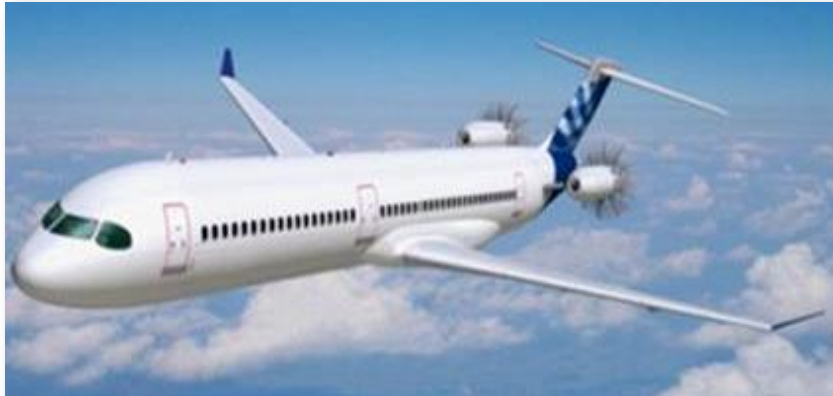
Figure 2. Airbus R&T concept study with rear mounted open rotor engines
